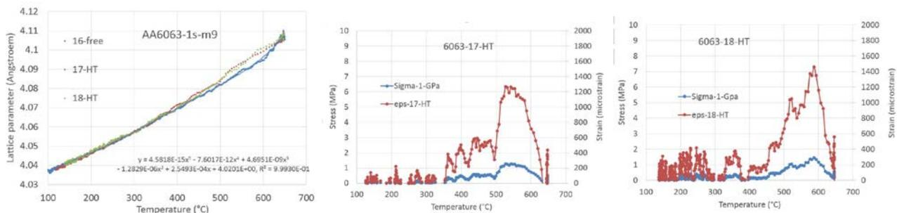
Fig. 3: left, lattice parameter during casting in a free to contract configuration and during constrained casting. Centre and right, elastic strain and longitudinal stress as a function of temperature for the two cracked AA6063 samples.
