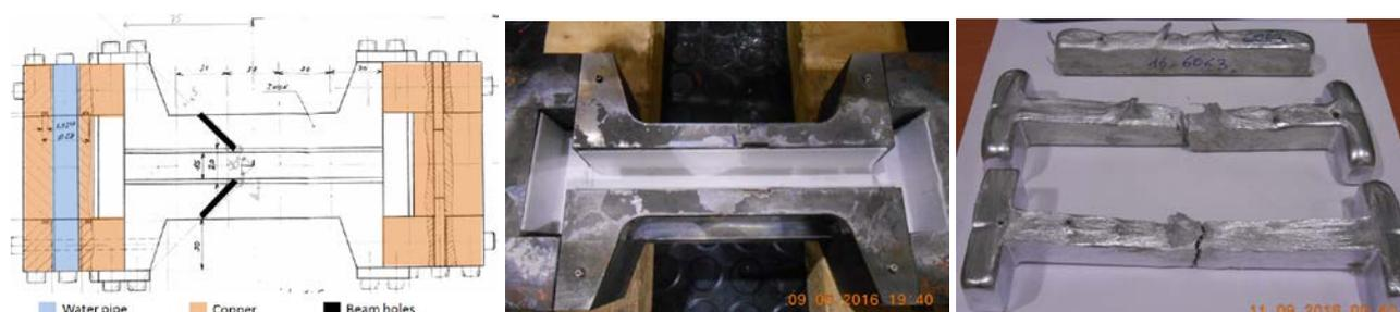
Fig.1: dog bone shape mould design (top view): two holes within the mould avoid neutron absorption by steel. Promat alumina foils prevent metal leakage through the holes. Centre: top view of dog bone shape mold with alumina foils in place. Right, 3 AA6063 samples, 2 dog bone samples and one free to contract samples.
