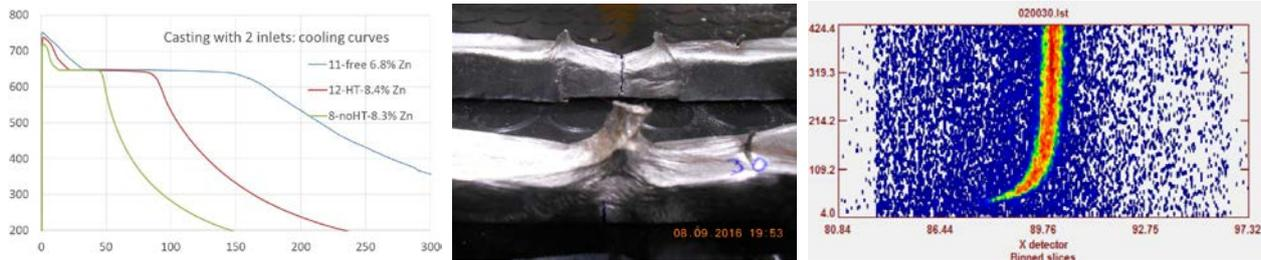
Fig.2: Left, temperature evolution during casting for 3 Al-Zn5% samples. Centre, AlZn5 cast with two inlets showing a hot tear and cast with one inlet showing no crack. Right, ND signal versus time (or temperature) with averaging over 9 periods.
