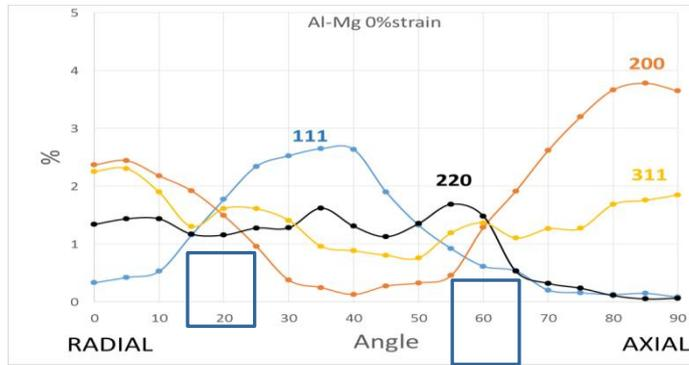
Figure 3. Diffracted intensity evolution of several hkl from radial to axial direction for the un-deformed Al-3%Mg alloy. These variations account for the initial texture of the alloy which is, in summary, described by a  $\langle 200 \rangle$  and  $\langle 311 \rangle$  fiber texture, with the fiber axes parallel to the extrusion axes direction.
