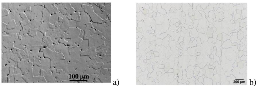
Figure 1. Pure aluminum a) and Al-Mg alloy b) grain size.
