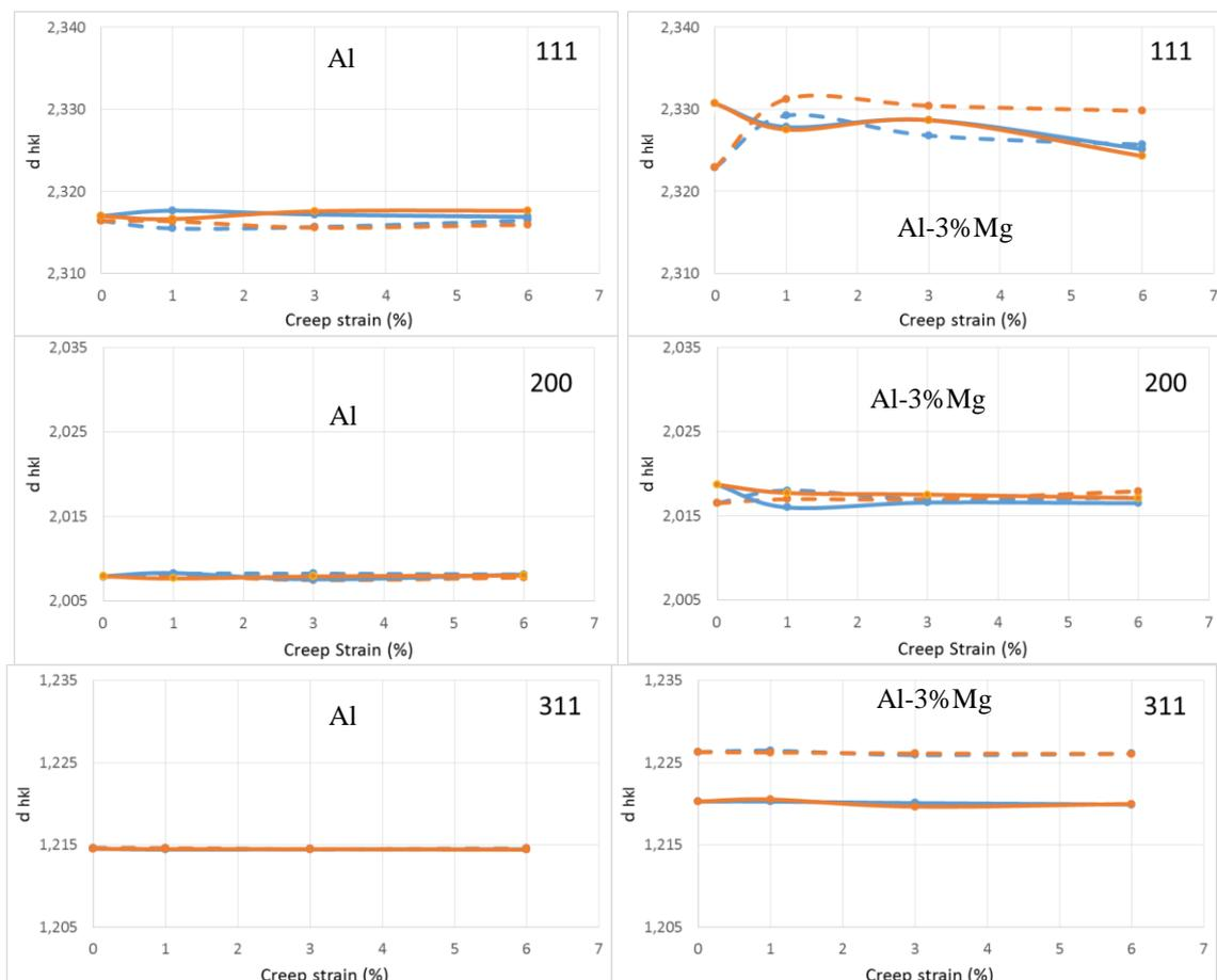
Figure 4.  $d_{hkl}$  for the pure Al and Al-3%Mg (111), (200) and (311) reflections. Axial(dashed lines) and radial directions are shown. 29MPa blue lines and 21MPa brown lines. Al plots area located to the left and Al-Mg to the right in the plot.
