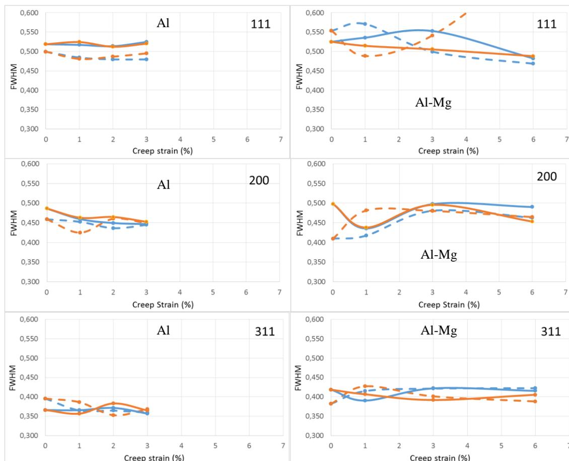
Figure 6. FWHM vs. creep strain for the materials investigated. Axial and radial directions are shown. 29MPa blue lines and 21MPa Brown lines. Al plots area located to the left and Al-3%Mg to the right in the plot. Axial components are represented by dashed lines.
