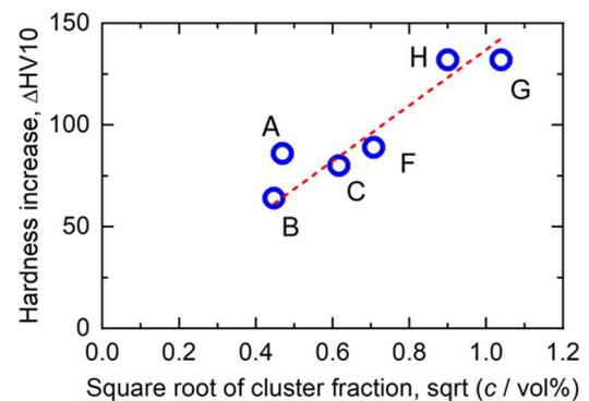
Fig. 5. Correlation between hardness increase and the square root of volume fraction of irradiation-induced clusters.
