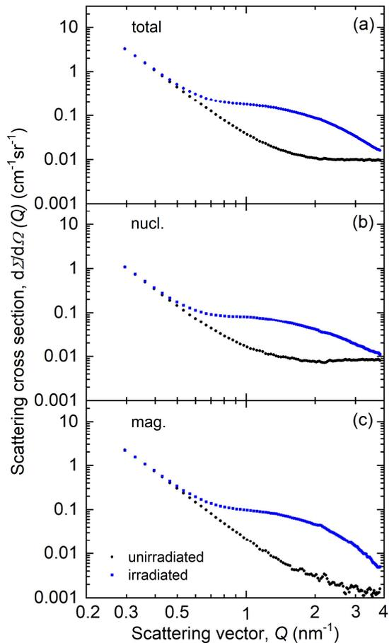
Fig. 2: Measured total (a), nuclear (b) and magnetic (c) scattering cross sections for the unirradiated reference and irradiated conditions of steel G.
