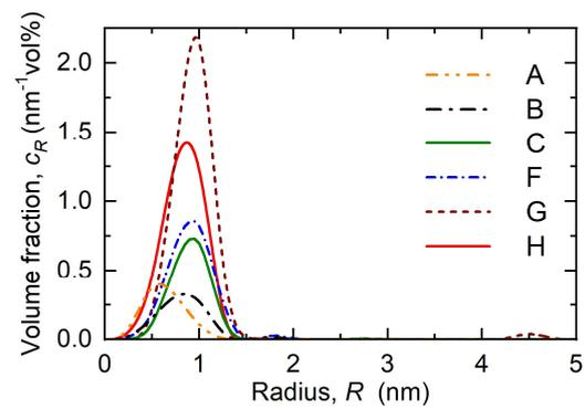
Fig. 4: Size distribution of irradiation-induced scatterers in terms of volume fraction per size increment for the steels, A, B, C, F, G and H.
