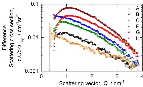
Fig. 3: Measured magnetic difference scattering cross sections of the steels A, B, C, F, G and H with the unirradiated condition subtracted.
