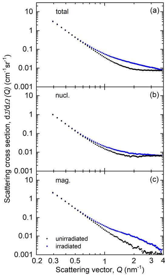
Fig. 1: Measured total (a), nuclear (b) and magnetic (c) scattering cross sections for the unirradiated reference and irradiated conditions of steel B.
