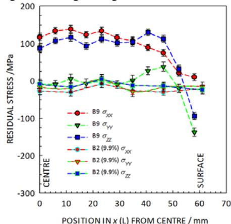
**Figure 2 Comparison of residual stresses remaining in a block cold compressed 9.9% (B2) and a block receiving no cold compression (B9) for a line scan in the longitudinal direction (x) of the blocks. (SALSA).**
