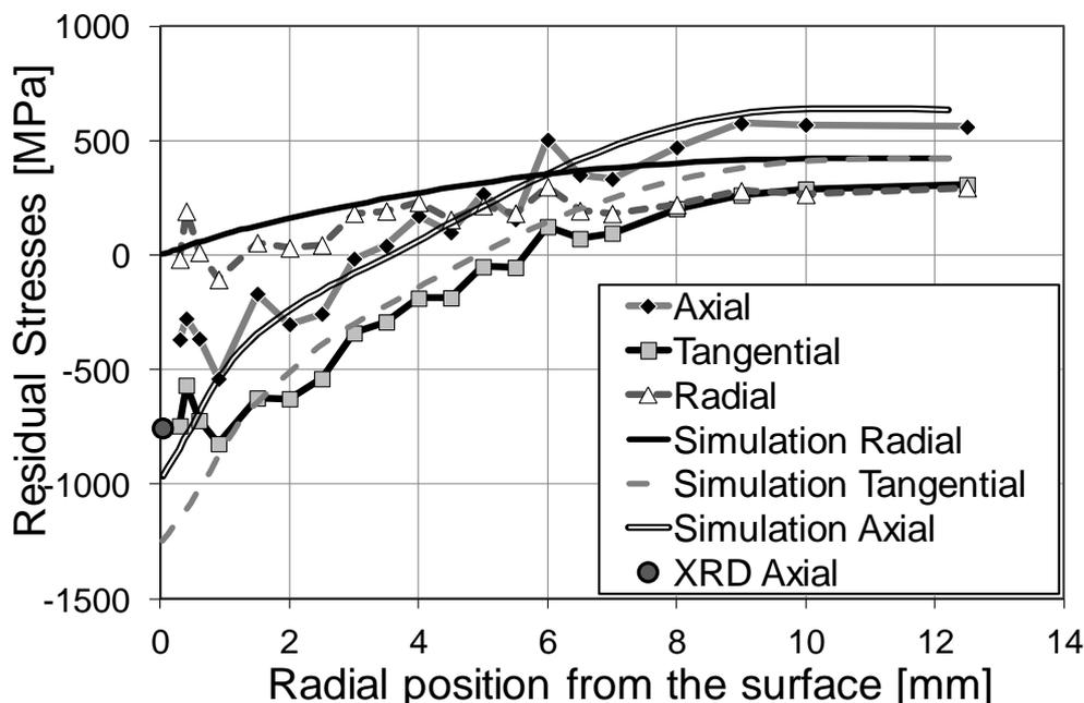
Figure 2: Distribution of triaxial residual stresses from the surface to the center of a cylinder made of C35 with  $\varnothing$  25 mm measured by neutron diffraction and calculated by FEM simulation
