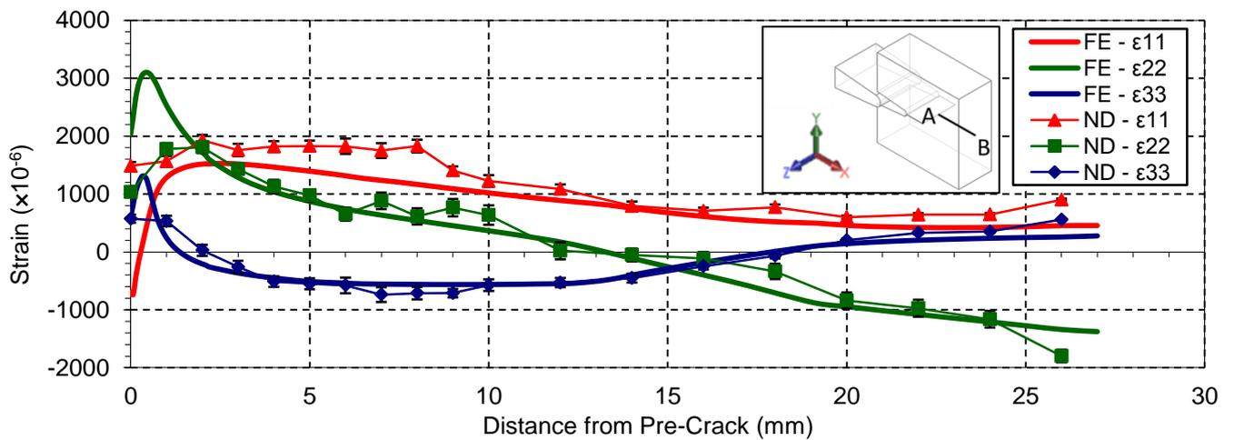
Figure 3 Comparison of residual strains measured along line A-B in WC(T)4 with FE predictions
