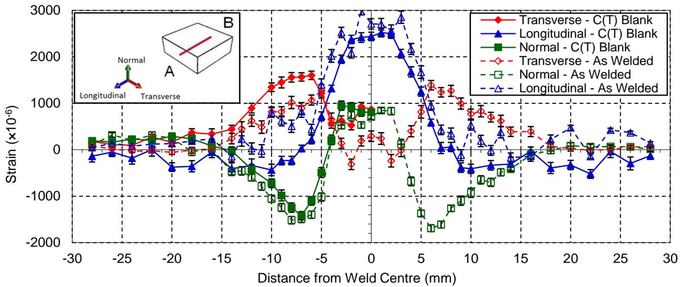
Figure 1 Comparison of residual stresses measured along line A-B in specimen EBW5 after welding and in C(T) blank
