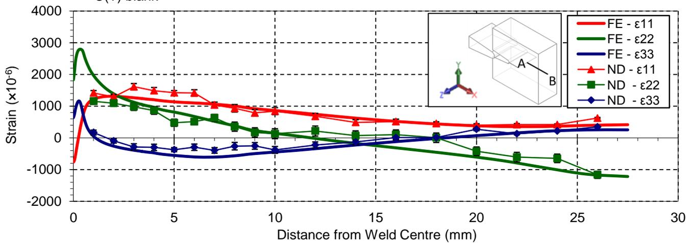
Figure 2 Comparison of residual strains measured along line A-B in WC(T)3 with FE predictions
