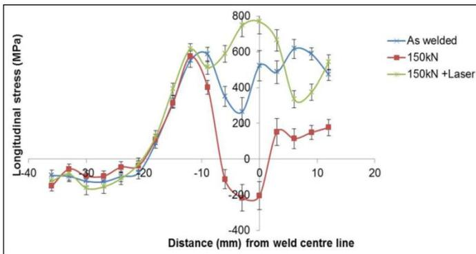
Fig. 2 – Residual stress profile across the weld in specimens with different processing conditions. Measured 2 mm below the top surface.
