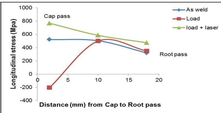
Fig. 3 – Variation of peak residual stress magnitude through the thickness of same specimens shown in fig. 2.
