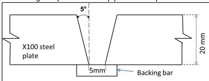
Figure 1: Pipeline steel plate set-up with backing bar
