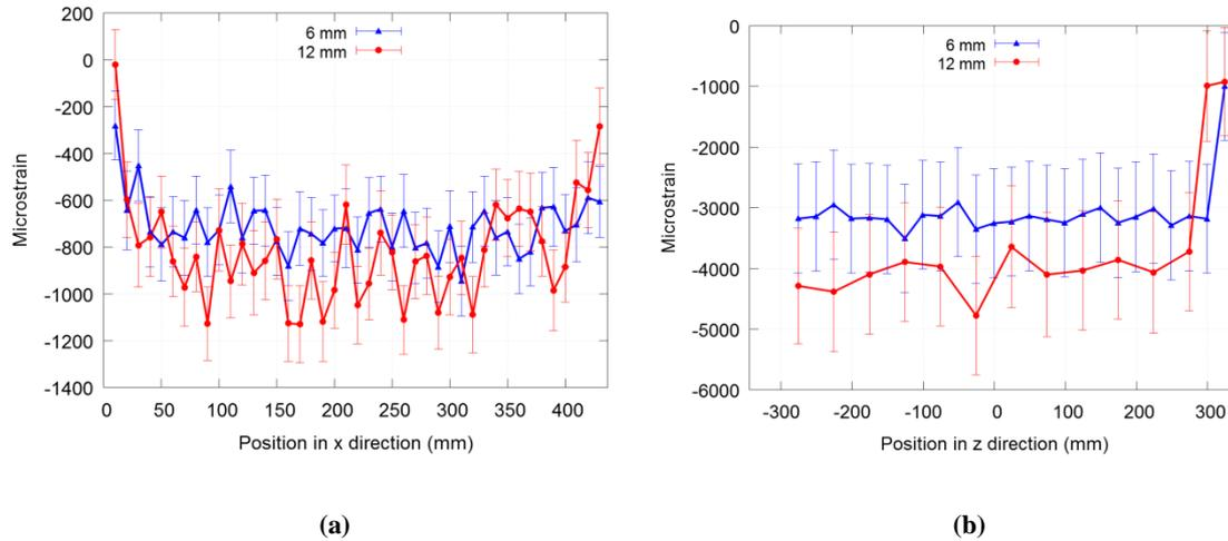
**Figure 1** : Results of strain measurements for a scan made along (a) a horizontal line on the larger surface of the ZB block based on  $(\bar{3}11)$  reflection and (b) a vertical line (the casting direction) on the larger surface of the ZS block based on  $(\bar{1}11)$  reflection.
