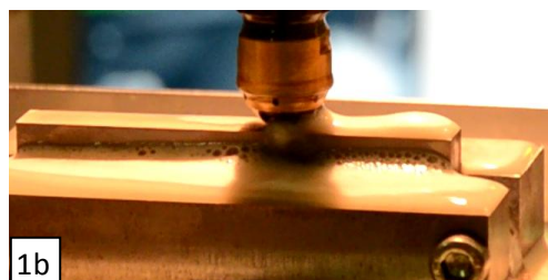
1b. Deep rolling tool on sample during processing
