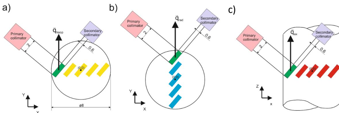
Fig. 1. Schematic set-up of the sample on SALSA beamline for a) hoop component; b) radial component; c) axial component.
