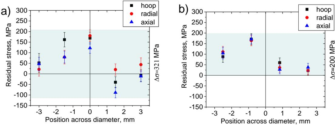
Fig. 2. Residual stress profile across the sample diameter for a) AB, b) HT.
