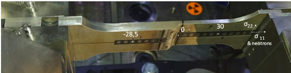
Figure 1: Specimen mounted in a tensile machine on SALS beamline.
