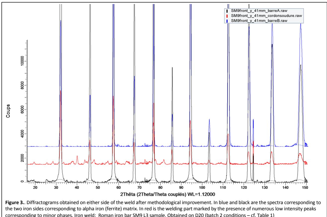
**Figure 3.** Diffractograms obtained on either side of the weld after methodological improvement. In blue and black are the spectra corresponding to the two iron sides corresponding to alpha iron (ferrite) matrix. In red is the welding part marked by the presence of numerous low intensity peaks corresponding to minor phases. Iron weld: Roman iron bar SM9 L3 sample. Obtained on D20 (batch 2 conditions – cf. Table 1)
