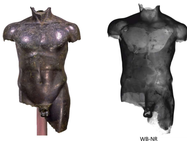
Figure 1. WB neutron radiography (stitched) of the statue from which all repairs were identified.
