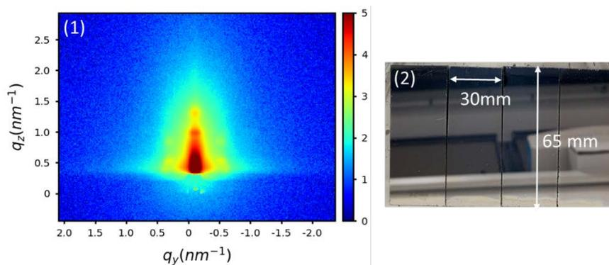
Fig 1(1) The GISAXS pattern of the mesoporous silica film using as templates; (2) The mesoporous silica film coted on Pt substrates.
