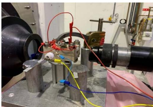
Fig 2 The experiment setup. The middle part is the designed cell connected to the potentiostat.
