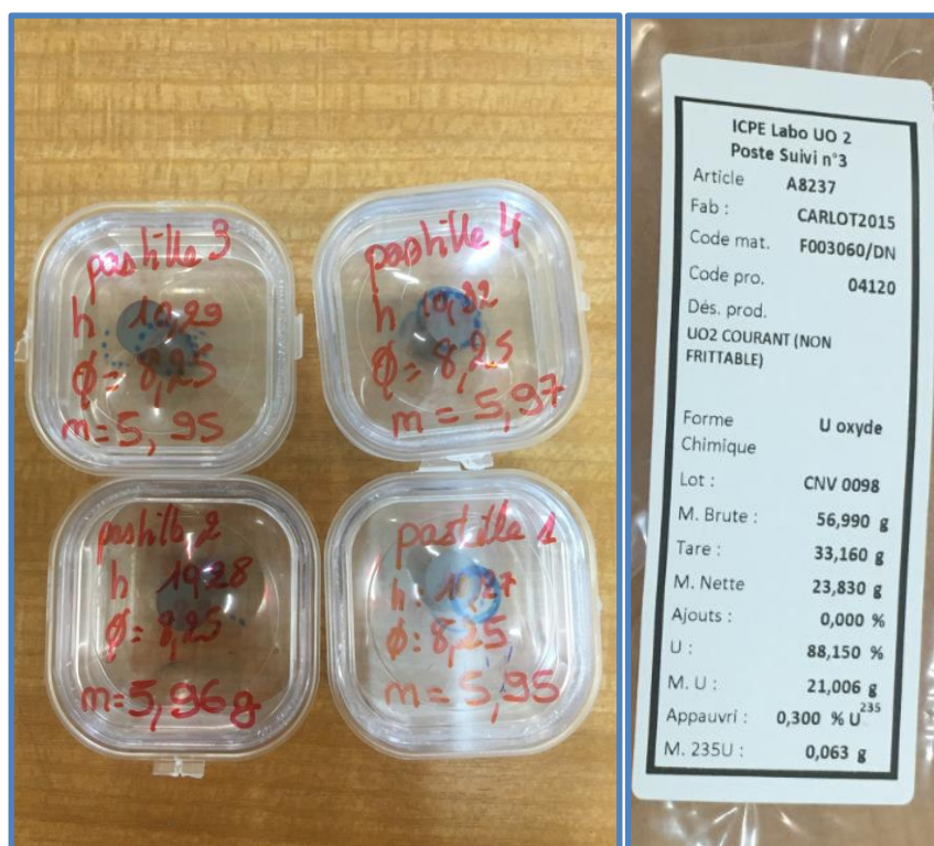
Fig. 1. Characteristics of the four UO 2 pellets
