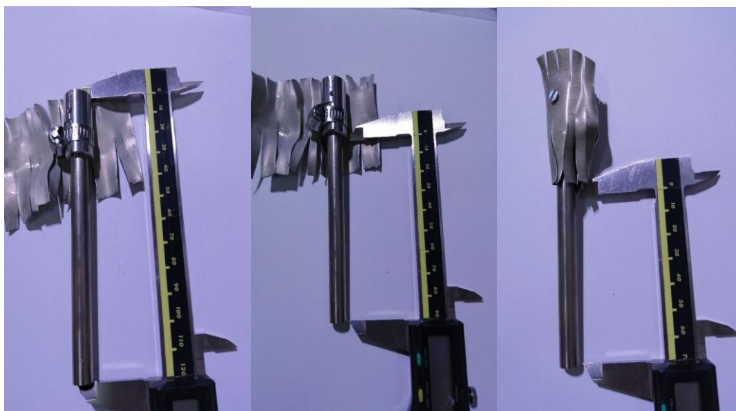
Fig. 1. \text{ThO}_2 sample in the ZrY4 container with its Al sample holder wrapped in a Cd foil.
