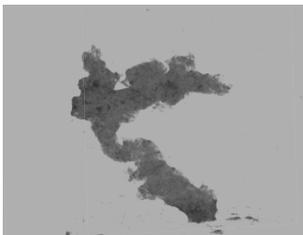
Figure 3. The final wormhole from conical experiment PIN44.
