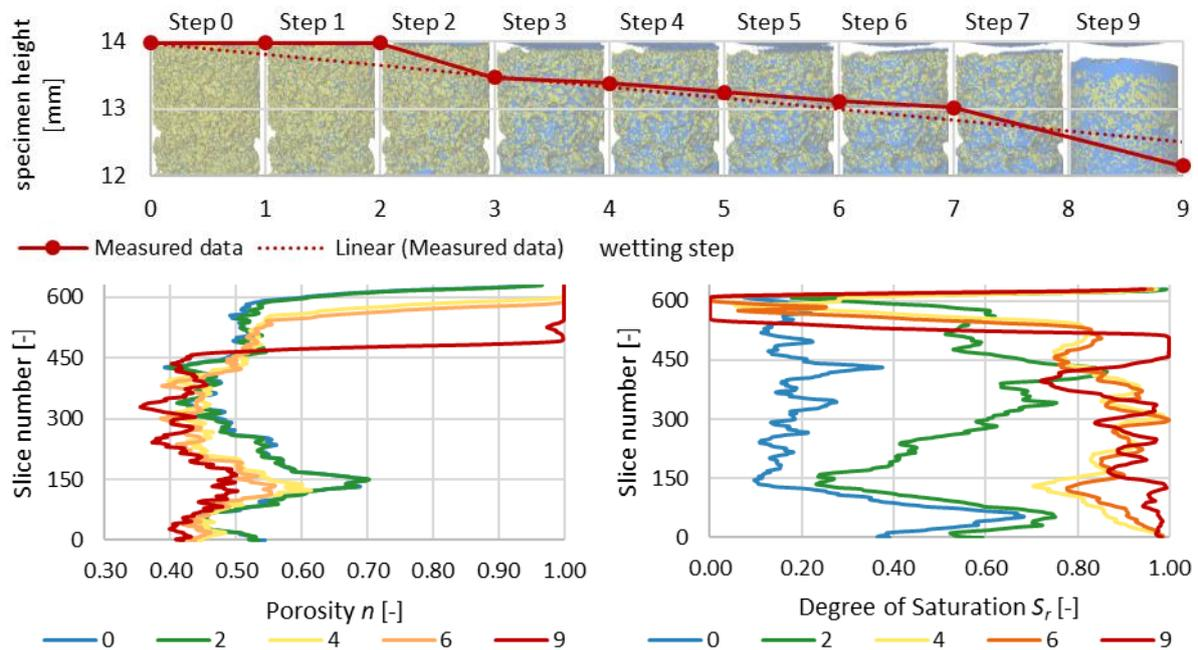
**Figure 2:** Development of the specimen height (top; Sand = yellow, water = blue, air = transparent) as well as the vertical porosity (bottom left) and the degree of saturation (bottom right) during the step-wise sample irrigation in experiment 3
