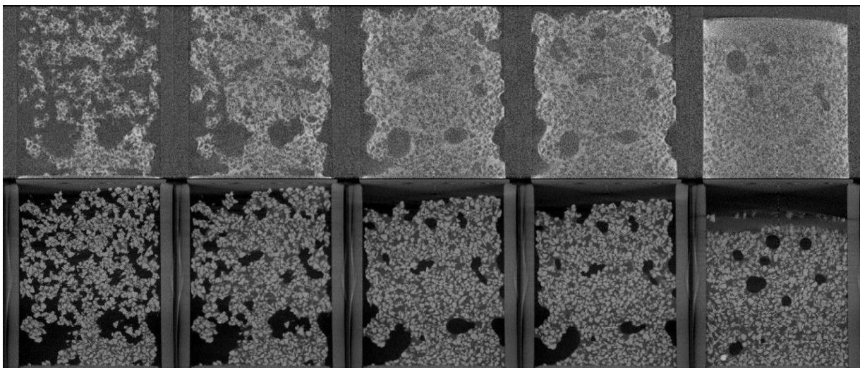
**Figure 1:** Central vertical slices obtained from neutron tomography (top) and X-ray tomography (bottom) during stepwise wetting through the specimen bottom (from left to right: image data of scans 0, 2, 4, 6 and 9)
