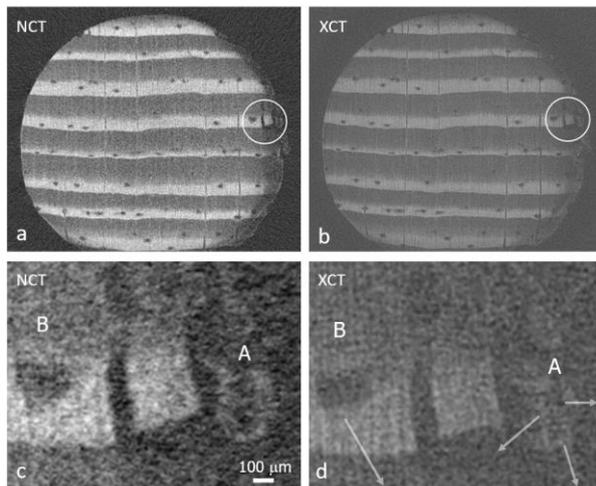
**Fig. 4:** Tomographic slices of raw data images: a) and b) cut planes of NCT and XCT, respectively. c) and d) show the regions marked in a) and b) zoomed in.
