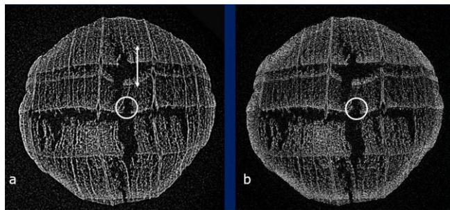
**Fig. 2** (a) NCT, (b) XCT of fully pyrolyzed beech wood dowels. Images are brightness/contrast adjusted for comparison.
