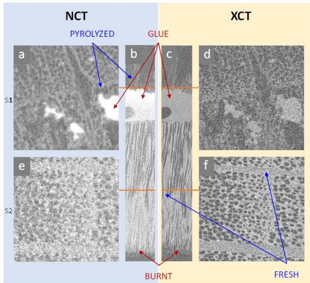
**Fig. 1** Overview panel of NCT and XCT (raw data images) of a fully pyrolyzed beechwood sample a) and d) showing corresponding horizontal sheets. b) and c) show axial sheets including the glued regions (white patches in NCT). d) and f) show parts from the pristine region of the partially burnt
