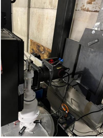
Figure 1: Left: Designed carbonation chamber mounted on NeXT. Right: Complete setup controlling CO 2 concentration and temperature inside the chamber.
