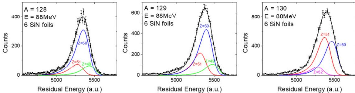
Fig. 2. Residual energy spectra of heavy-fragment masses at 88 MeV energy in  $^{239}\text{Pu}(n_{\text{th}}, f)$  penetrating 6  $\mu\text{m}$  of SiN degrader, from  $A = 128$  to  $A = 130$ , with their individual Z constituents. The asymmetric peak profile was determined in a calibration measurement with stable ions (see text).
