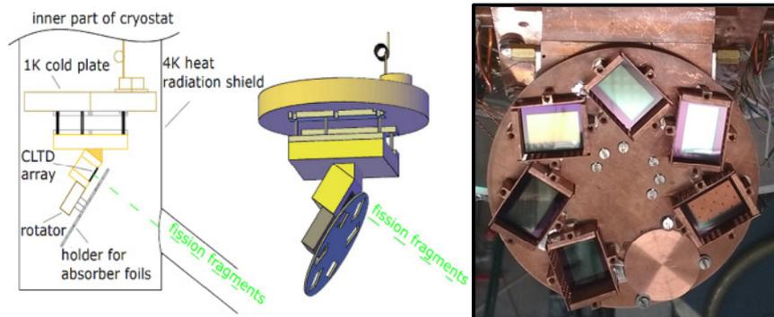
Fig. 1. Schematic view of the detector cryostat with rotatable sample changer for silicon nitride absorber stacks in front of the CLTD's as residual-energy detector (left). Front view of the rotator disc (right). One position is occupied by a calibration  $\alpha$  source.
