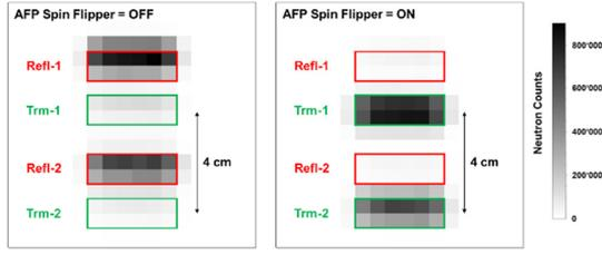
Fig. 2 Detector counts in 10 seconds at a wavelength of 0.48 nm for the two adiabatic spin flip device states (off and on). The detector has an active area of  $100 \times 100 \text{ mm}^2$  divided into  $16 \times 16$  pixels. The two beams cause four beam spots behind the spin analyzer – reflected (red box) and transmitted (green box) beam of the upper and lower beam, respectively. The employed detector was purchased by the company CDT.
