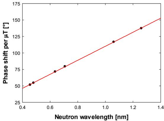
Fig. 5 Phase shift per one microtesla as a function of the neutron wavelength (of the upper beam).
