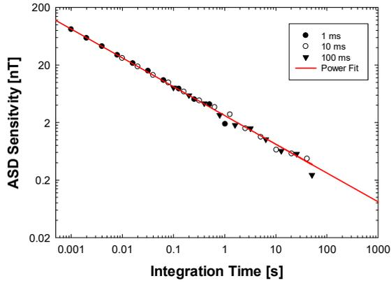
Fig. 4 ASD plot of the stability/sensitivity of our Ramsey apparatus as a function of the measurement/integration time. The red line indicates the improvement in sensitivity due to Poisson statistics.
