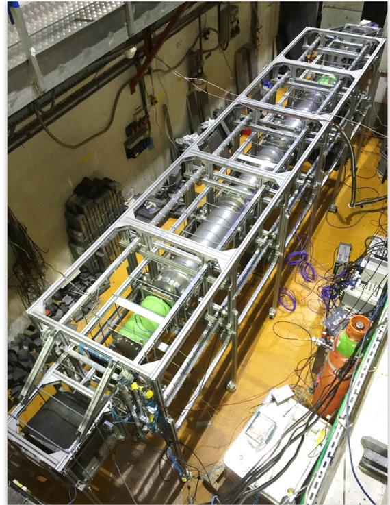
*Fig.1 Installation of the Beam EDM prototype experiment at the PF1b beam line at ILL. The length of the setup is approximately seven meters. The neutron beam exits the wall at the experimental site in the lower left corner of the image. The high-rate neutron detector is located at the upper right corner of the image. The green coils are the neutron resonance spin flippers. They are separated by 4 m. Between the coils the 3.5 m long aluminum vacuum pipe is installed.*
