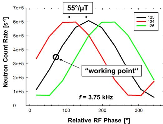
Fig. 4 Ramsey phase-scan at 3.75 kHz for three different static magnetic field setting of 124, 125, and 126  $\mu\text{T}$ . The phase shift of the sinusoidal pattern is about  $55^\circ/\mu\text{T}$ .
