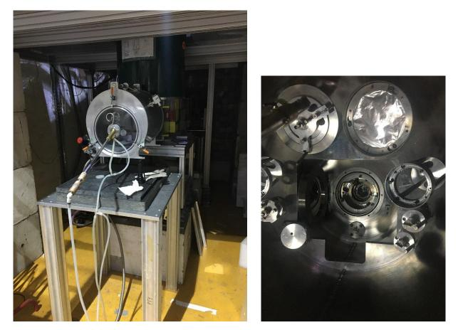
Photographs of the experiment taken during installation. Left: the magnet with attached service chamber for exchange of the beam stop in the center of the magnet (normally it is used for exchange of samples in that location). In the final configuration of the experiment, the detector and its shielding were located on the table behind the magnet. Right: view into the service chamber; the various tools surround the central bore giving access to the magnet.
