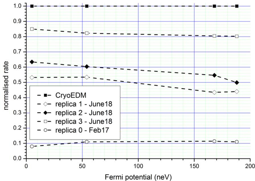
Figure 3: The count rates of the three replica guides normalised to that of the cryoEDM guide. The second batch of replica guides (June18) shows a substantial improvement to that of the first replica guide (Feb17) with transmissions approaching that of the cryoEDM guide.
