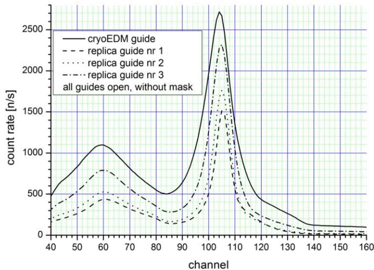
Figure 1: The neutron count-rate as recorded by the large area detector for the three replica guides and the cryoEDM guide installed in the chamber. The plots show data taken with the detectors all operating in the "open" configuration without a mask.
