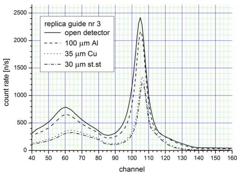
Figure 2: The neutron count rates as recorded by the large area detector with replica guide nr. 3 installed in the chamber. The detector has been equipped with an Al, Cu and stainless steel mask to obtain the transmission as function of a varying cut-off energy.
