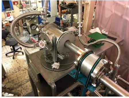
Fig.2 View of the installation at the UCN beam PF2 EDM and the scheme of the experiment. 1 — the chamber for preliminary cleaning of the UCN spectrum, 2 — main chamber with the sample.
