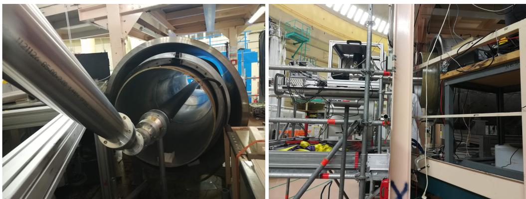
**Figure 1.** Pictures of the setup at the nEDM beamline. Left: Picture of the beamguide entering the main coil. The geometry on this side was constrained by the available space on the platform. Right: the beamguide exiting the main coil and the detector standing on a custom-made extension of the PF2 platform.
