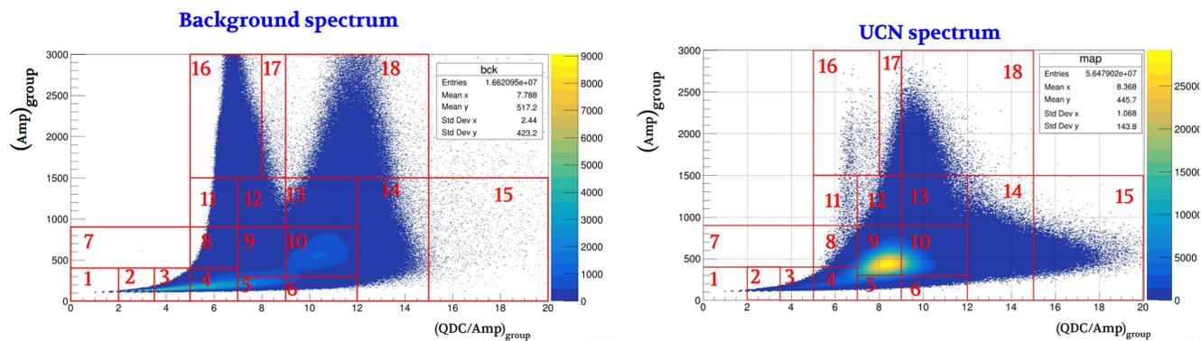
**Figure 2.** Pulse shape analysis based neutron/background selection, status as of January 2021. The upper figure shows a "background spectrum" taken with only CF<sub>4</sub> inside the detector, while the lower picture shows a similar measurement taken with CF<sub>4</sub>+He<sup>3</sup> inside the detector.
