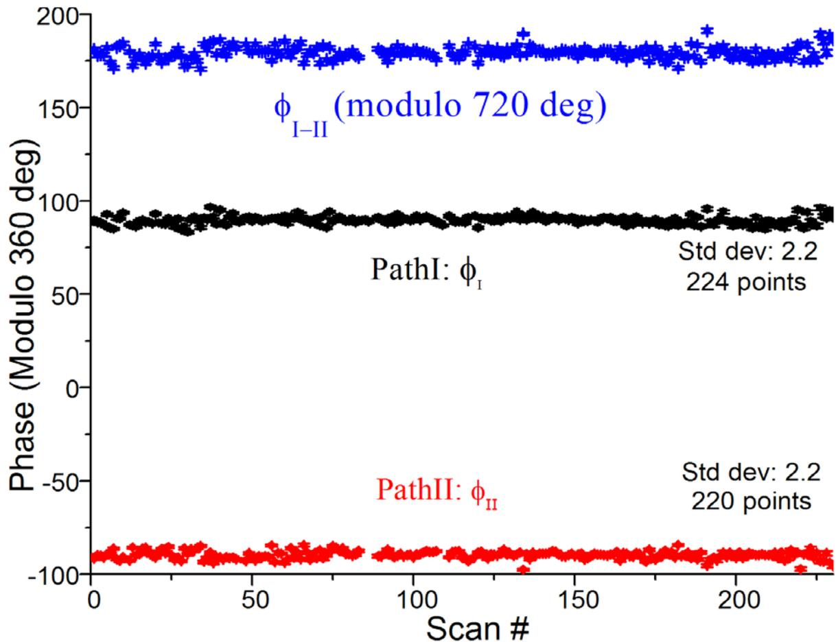
Fig.3 Observed IN-OUT phases with the nondispersive dual sample placed in path I and path II.
