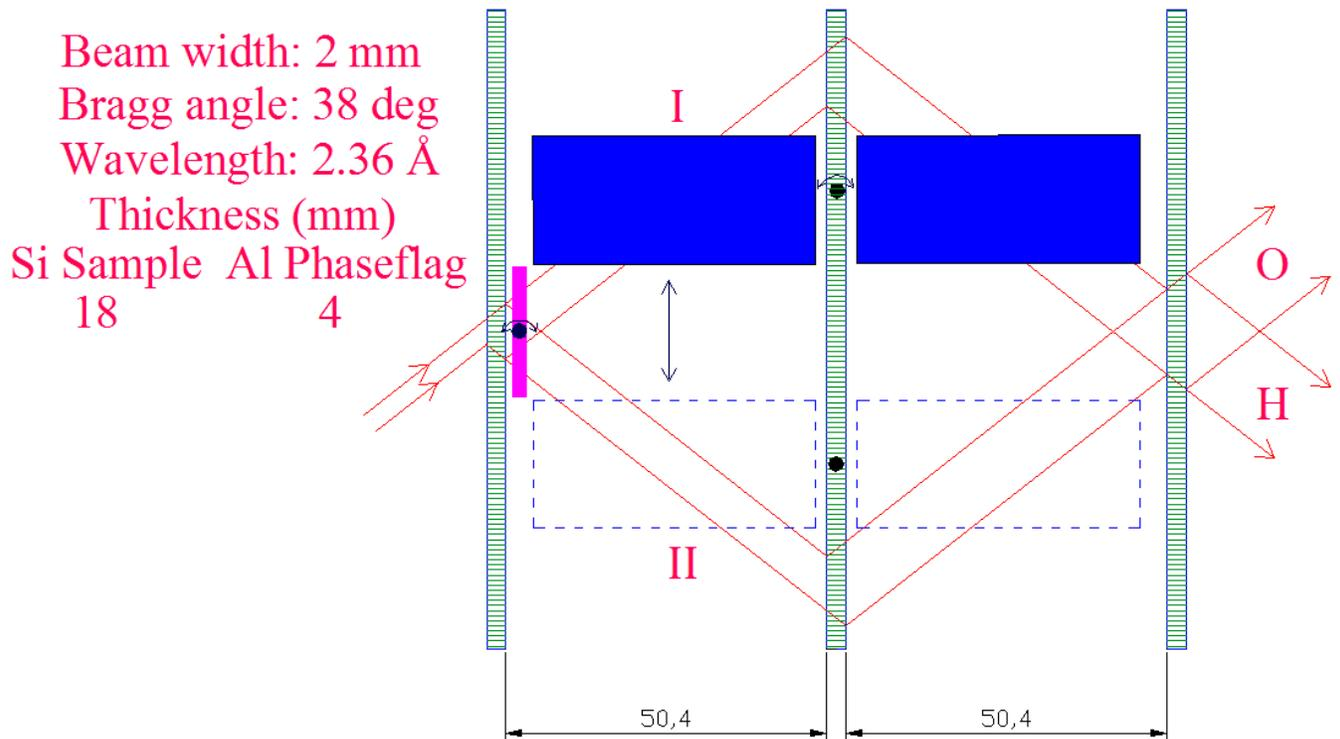
Fig.1 High precision  $b_c$  determination (schematic) employing a thick dual nondispersive sample in a large symmetric LLL interferometer.
