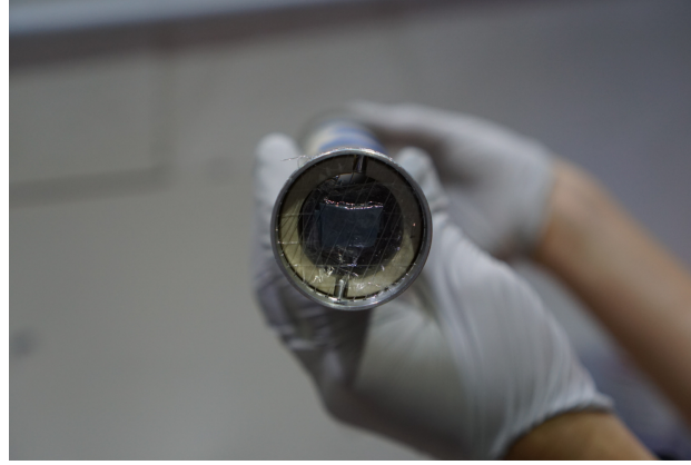
Picture of the ^{192}\text{Os} powder target contained in a plastic bag.
