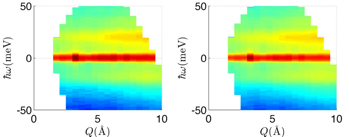
Figure 1:  $Q, \omega$  maps at 200 K (left) and 400 K (right) measured with an initial neutron energy  $E = 65$  meV. The scattered intensity is given on a logarithmic color scale.
