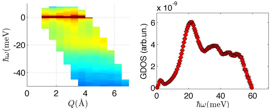
Figure 2: Left:  $S(Q, \omega)$  measured at 400 K with an initial neutron energy  $E = 14\text{ meV}$ . Right: Generalized density of phonon states measured at 400 K with an initial neutron energy  $E = 65\text{ meV}$ .
