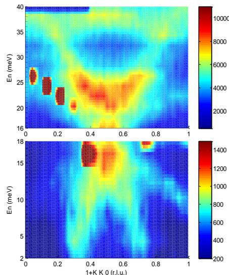
**Fig. 1** Neutron scattering intensity maps of the magnetic excitation spectrum of  $\text{La}_{1.62}\text{Sr}_{0.38}\text{CoO}_4$ .
