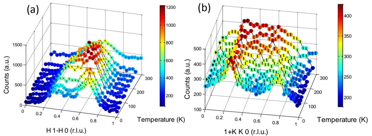
**Fig. 2** Temperature dependence of the hour-glass dispersion (a) Temperature dependence of constant energy-scans at 5 meV. (b) Temperature dependence of constant energy-scans at 30 meV.
