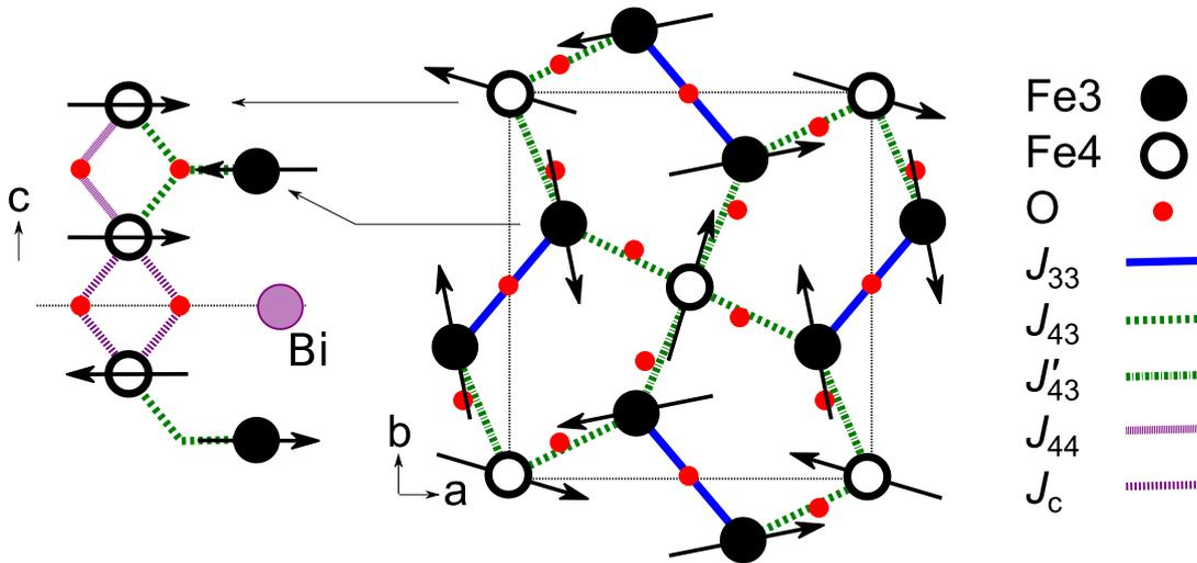
Figure 1. The crystal structure of  $\text{Bi}_2\text{Fe}_4\text{O}_9$  showing only the  $\text{Fe}^{3+}$  ions in the Cairo pentagonal lattice, including the three-fold sites (solid circles) and four-fold sites (open circles) and the exchange interactions.
