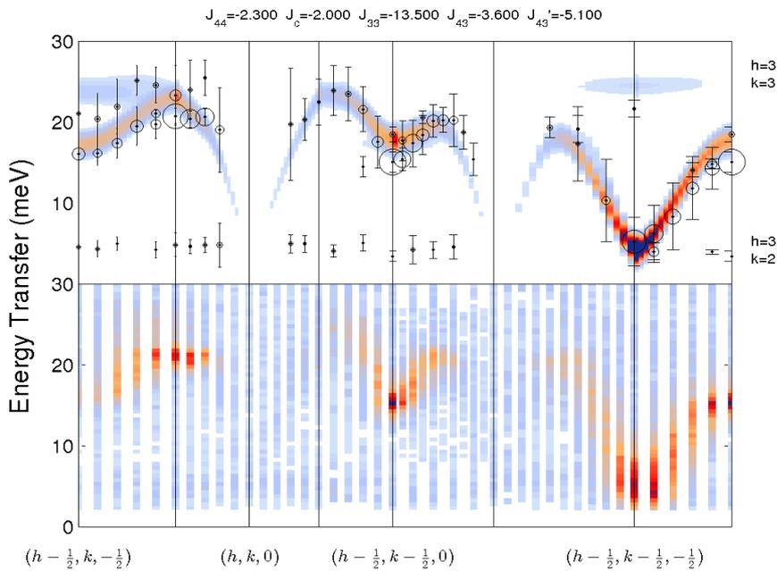
Figure 2. (Top) Simulated magnon dispersion with fitted peak positions and widths as errorbars. (Bottom) Measured constant  $q$  scans with intensity on a colour scale. One dispersive magnon branch is clearly seen, with a flat optic phonon mode around 5 meV.
