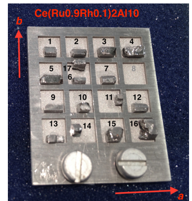
Fig. 1. Sample mount with 16 co-aligned single crystals, for a total of 611 mg.
