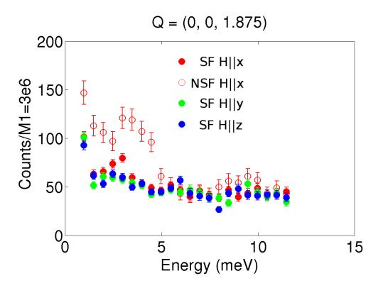
Energy scan at Q = (0, 0, 1.875) where a broadening of the magnetic excitation was reported with respect to Q = (0, 0, 1.225). The NSF channel with H||x clearly shows a phonon, while the magnetic scattering, fully visible in the SF channel with H||x, appears at lower energy than the phonon. Phonon and magnetic scattering would appear superposed in unpolarised data like those shown in [Zaliznyak PRL 87, 017202 (2001)].
