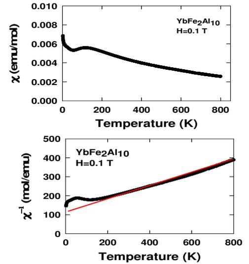
**Figure 1:** Temperature dependent  $\chi$  of YbFe<sub>2</sub>Al<sub>10</sub> sample used in our IN4 experiment.
