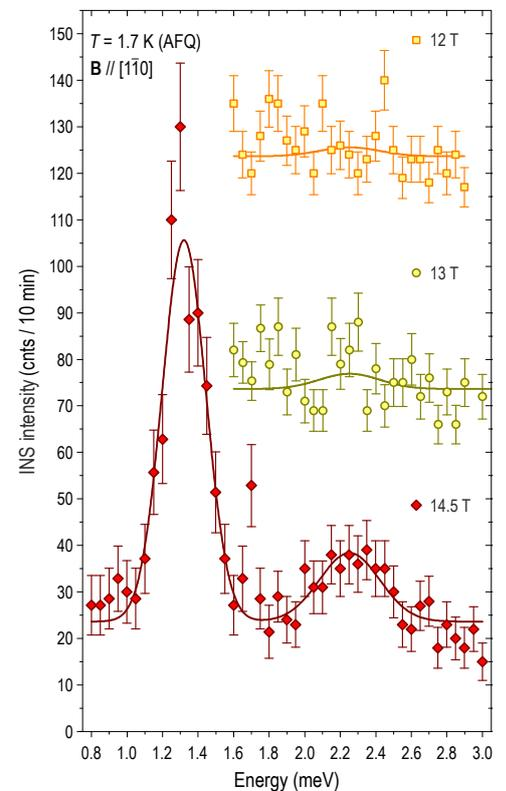
Fig. 1: INS spectra measured at Thales, near the zone center  $\Gamma(110)$ , which shows the appearance of the second resonance. The spectra are shifted vertically for clarity
