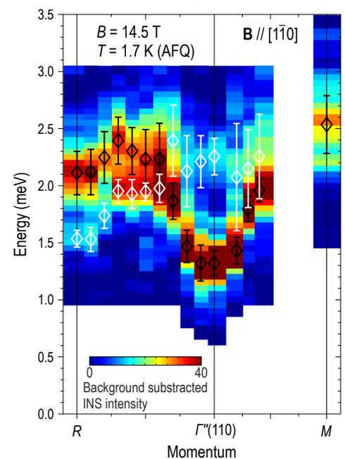
Fig. 2: Energy-momentum profile, which shows dispersion of the magnon spectrum along straight segments connecting the  $R(\frac{1}{2} \frac{1}{2} \frac{1}{2})$ ,  $\Gamma(110)$ ,  $M(\frac{1}{2} \frac{1}{2} 0)$  points.
