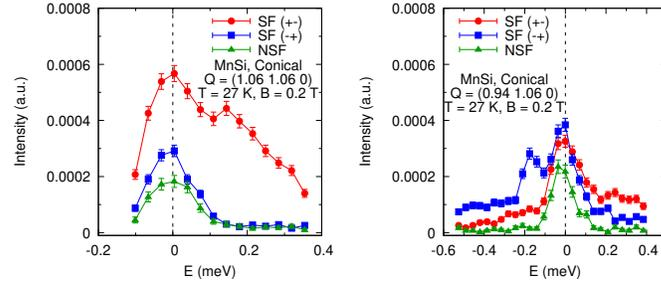
Figure 5. Polarized energy scan at  $\mathbf{Q}_{\parallel,2} = (1.06 \ 1.06 \ 0)$  and  $\mathbf{Q}_{\perp} = (0.94 \ 1.06 \ 0)$  in the conical phase [1, 2]. The first scan depicts the non-reciprocal dynamics. The second one shows the onset of the discrete helimagnon bands. We very recently published these results [3].
