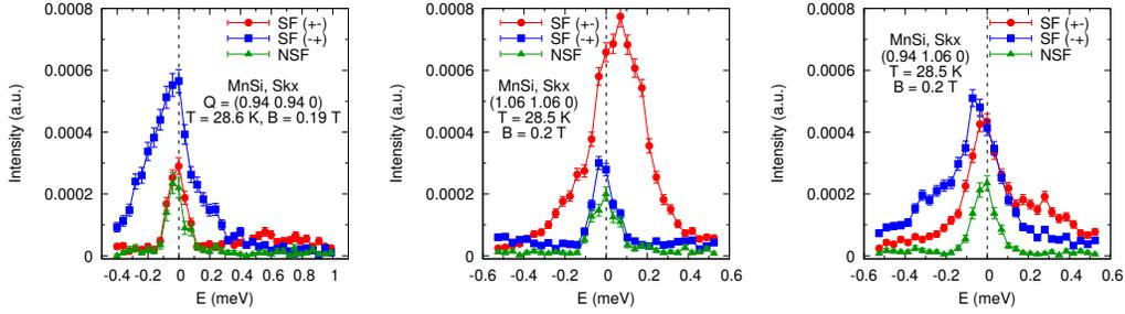
Figure 4. Polarized energy scan at  $\mathbf{Q}_{\parallel,1} = (0.94 \ 0.94 \ 0)$ ,  $\mathbf{Q}_{\parallel,2} = (1.06 \ 1.06 \ 0)$  and  $\mathbf{Q}_{\perp} = (0.94 \ 1.06 \ 0)$  in the skyrmion phase. The first two scans show the non-reciprocal dynamics. The third one the ensuing continuum of states. The following figures show the same scans in the other magnetic phases.
