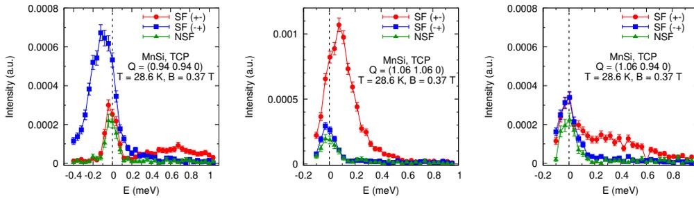
Figure 7. Polarized energy scan at  $\mathbf{Q}_{\parallel,1} = (0.94 \ 0.94 \ 0)$ ,  $\mathbf{Q}_{\parallel,2} = (1.06 \ 1.06 \ 0)$  and  $\mathbf{Q}_{\perp} = (1.06 \ 0.94 \ 0)$  at the tri-critical point [9]. The first two scans exhibit non-reciprocal dynamics similar to the conical and skyrmion phase. The third scan shows a broad spectrum of excitations.
