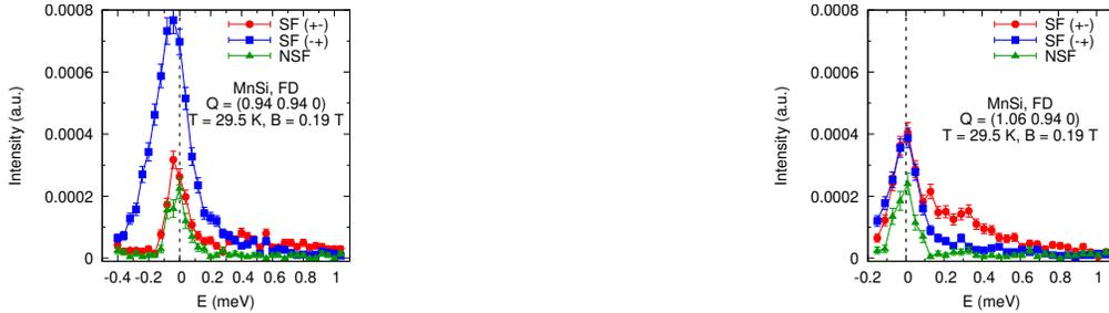
Figure 6. Polarized energy scan at  $\mathbf{Q}_{\parallel,1} = (0.94 \ 0.94 \ 0)$  and  $\mathbf{Q}_{\perp} = (1.06 \ 0.94 \ 0)$  in the fluctuation-disordered phase [7]. The first scan exhibits a similar non-reciprocity as observed in the conical and skyrmion phase, albeit shifted towards lower absolute energies. Low-energy excitations can be detected in the second scan.
