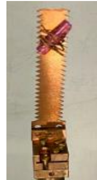
Figure 2: Single crystal of Er 2 Si 2 O 7 on a copper mount with ( hk 0) horizontal.
