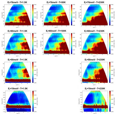
To go further, imaginary part of the magnetic susceptibility  $\chi''$  can be calculated. One can also perform temperature difference between low and high temperatures.
