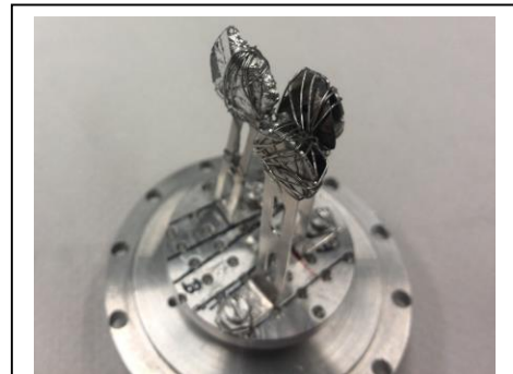
Fig. 1 Foto of the three coaligned three large crystals with a total mass of 4.7 g
