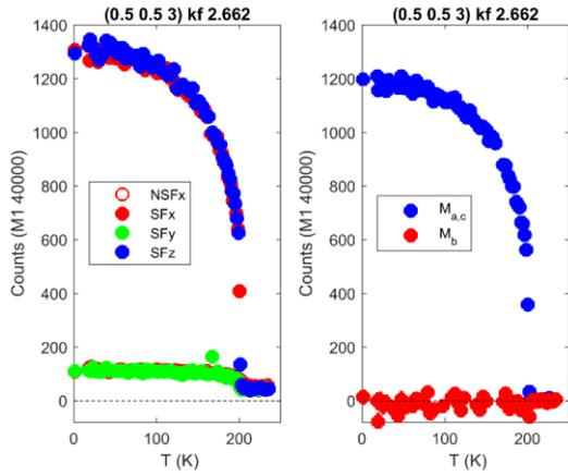
**FIG. 1** : Polarization analysis of the (0.5 0.5 3) reflection on IN20. All the static signal goes into the  $M_{a,c}$  component as expected. The small  $SF_y$  signal stems from the finite though quite large Flipping ratio of  $\sim 25$  (determined at (112)).
