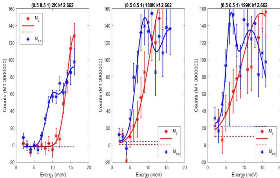
**FIG. 3** : Temperature dependence of the polarized signals at (0.5 0.5 1). The gap in c-polarized magnetic fluctuations only modestly decreases upon approaching the Néel temperature. The b polarized excitations also soften or become broader in energy.
