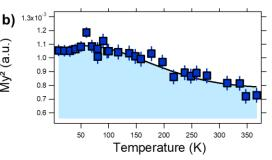
Figure 1: Temperature dependence of (a) the out-of-plane  $Mz^2$  and (b) in-plane  $My^2$ magnetic components as extracted from XYZ polarization analysis at  $\tau = 0$  ns. (c) Rocking scans around Q = (0.71,0,0) and (0.24,0,0) at T = 120 K. The data were collected on *IN11-C*.
