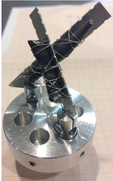
Figure 1: Co-aligned single crystal rods of CeAl 2 used in the present experiment.
