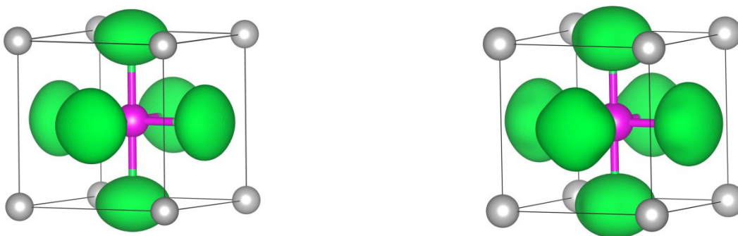
Fig. 3. Detail of the structure of \text{BaLiF}_{3-x}\text{O}_x at 400 °C (left) and 640 °C (right) with isosurface plot of anion PDF. Ellipsoids of 90% probability; PDF isovalue: 10^{-4} \text{ \AA}^{-3} (for color key, cf. Fig. 1).
