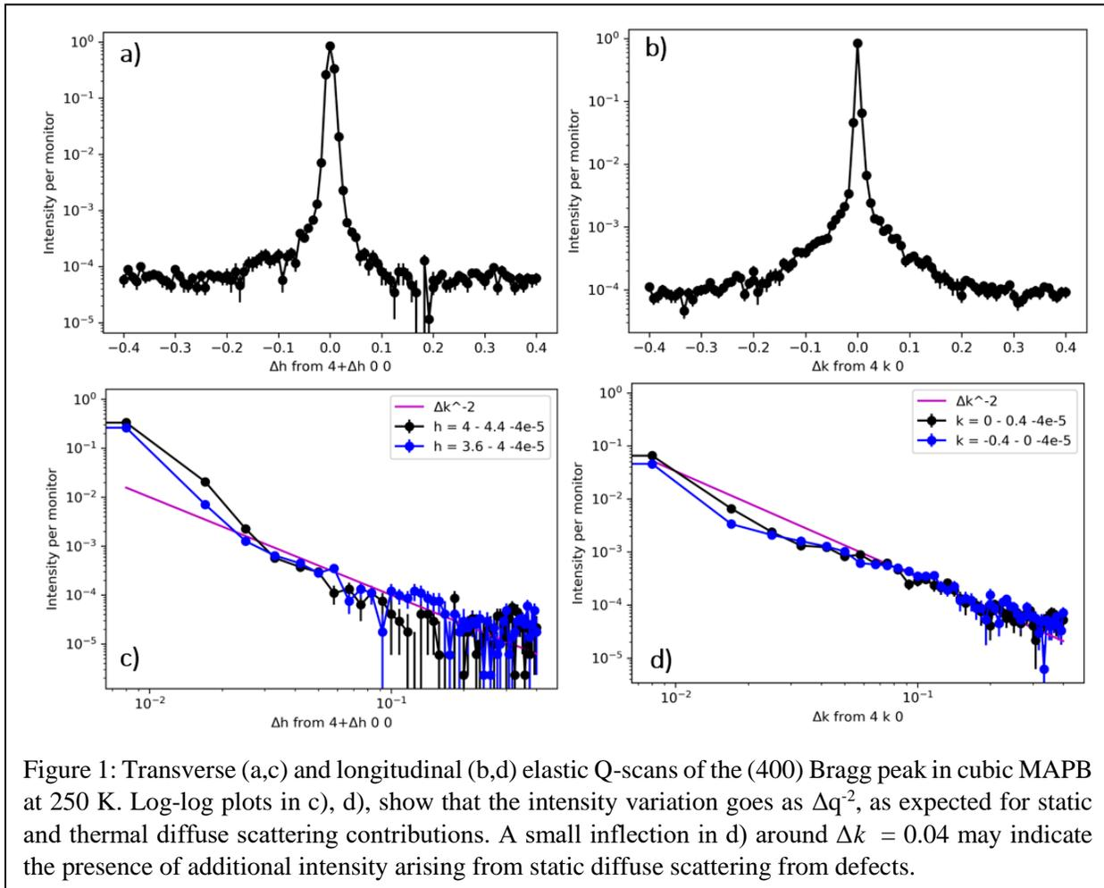
Figure 1: Transverse (a,c) and longitudinal (b,d) elastic Q-scans of the (400) Bragg peak in cubic MAPB at 250 K. Log-log plots in c), d), show that the intensity variation goes as  $\Delta q^{-2}$ , as expected for static and thermal diffuse scattering contributions. A small inflection in d) around  $\Delta k = 0.04$  may indicate the presence of additional intensity arising from static diffuse scattering from defects.
