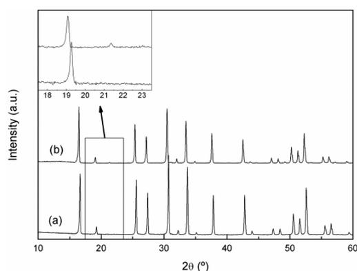
Fig. 1. XRD patterns of  $\text{Li}_7\text{La}_3\text{Zr}_2\text{O}_{12}$  after aging a) at 300 °C, b) at RT
