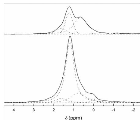
Fig. 2.  $^6\text{Li}$ -NMR spectrum of  $^6\text{Li}_7\text{La}_3\text{Zr}_2\text{O}_{12}$  (bottom) and aged at RT.
