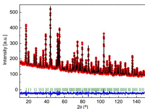
Fig. 3. NPD data of c150-LLZO at 77K. The points are the experimental data and the continuous curve the result of the refinement in the  $I\bar{4}3d$  sg. The bottom curve represents the difference between the experimental data and the calculated pattern.
