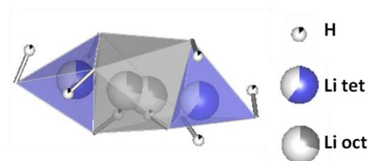
Fig. 6. Schematic representation of the lithium and proton sites resulting from the refinement of the NPD patterns of c350-LLZO within the  $Ia\bar{3}d$  space group.
