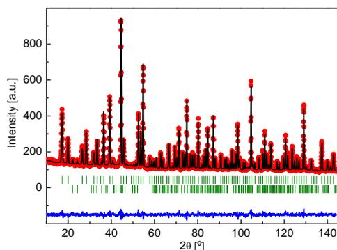
Fig.5. NPD data of c350-LLZO at 77K. The points are the experimental data and the continuous curve the result of the refinement within the  $Ia\bar{3}d$  sg.  $\text{Li}_2\text{CO}_3$  was included in the refinement as second phase.
