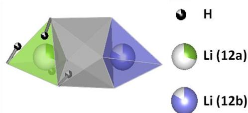
Fig. 4. Schematic representation of the lithium and proton sites resulting from the refinement of the NPD patterns of c150-LLZO within the  $I\bar{4}3d$  space group.
