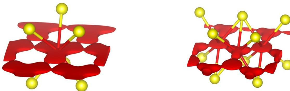
**Fig. 3.** Detail of the structure of  $\text{Na}_{0.5}\text{TiS}_2\text{-}3R_1$  (left) and  $\text{Na}_{0.9}\text{TiS}_2\text{-}2H$  (right) at 600 °C with isosurface plot of sodium PDF for  $F = 0.003 \text{ \AA}^{-3}$  (red:  $\text{Na}^+$ , yellow:  $\text{S}^{2-}$ ; ions with arbitrary radius).
