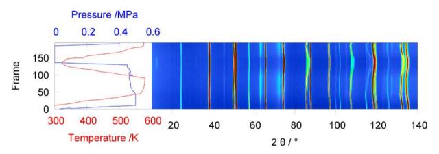
**Figure 1:** *In situ* powder neutron diffraction of LaGa<sup>2</sup> in a sapphire single-crystal cell showing the formation and decomposition of LaGa<sup>2</sup>D<sub>x</sub>. One frame equals two minutes. For this plot the NUMORs 144925-145119 were used [3].
