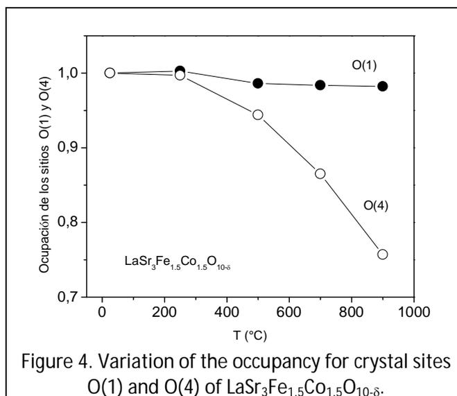
Figure 4. Variation of the occupancy for crystal sites O(1) and O(4) of LaSr<sub>3</sub>Fe<sub>1.5</sub>Co<sub>1.5</sub>O<sub>10-δ</sub>.
