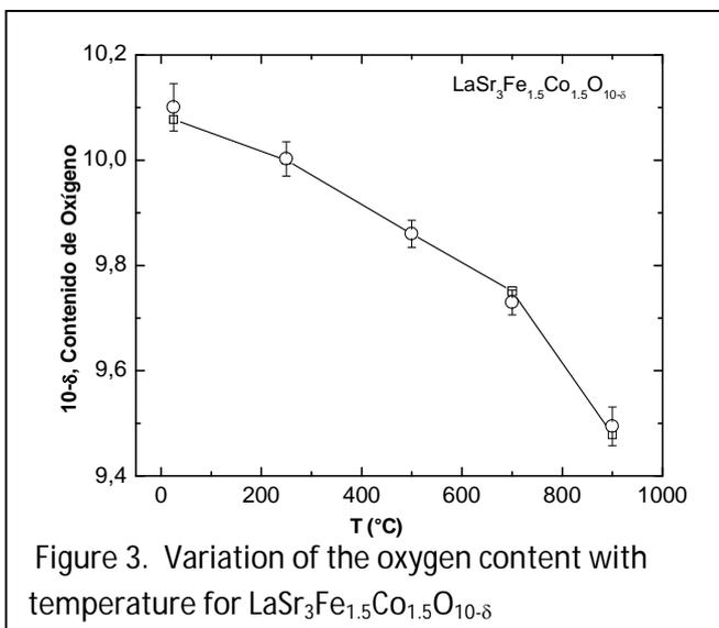
Figure 3. Variation of the oxygen content with temperature for LaSr<sub>3</sub>Fe<sub>1.5</sub>Co<sub>1.5</sub>O<sub>10-δ</sub>
