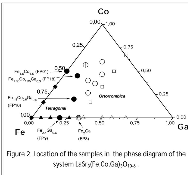
Figure 2. Location of the samples in the phase diagram of the system LaSr<sub>3</sub>(Fe,Co,Ga)<sub>3</sub>O<sub>10-δ</sub>.
