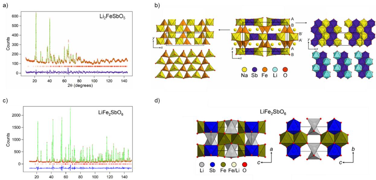
**Figure 1.** Observed, calculated and difference plots from the structural and magnetic refinement of  $\text{Li}_2\text{FeSbO}_5$  (a) and  $\text{LiFe}_2\text{SbO}_6$  (c) against NPD data collected at room temperature. Crystal structure of b)  $\text{Li}_2\text{FeSbO}_5$  and d)  $\text{LiFe}_2\text{SbO}_6$ .
