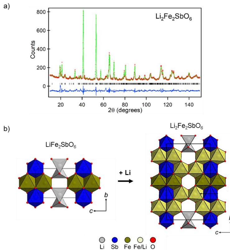
**Figure 2.** a) Observed, calculated and difference plots from the structural and magnetic refinement of  $\text{Li}_2\text{Fe}_2\text{SbO}_6$  against NPD data collected at room temperature. b) Crystal structure modification while Li deintercalation in  $\text{Li}_x\text{Fe}_2\text{SbO}_6$ .
