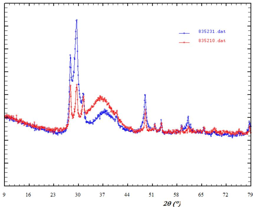
**Figure 3:** Transition of glassy  $\text{NaCl}\cdot 10.2\text{D}_2\text{O}$  at 150 K (red, with a contaminant of ice Ih) into ice Ic plus a remaining amorphous solid with higher salt concentration (blue). Note the shift of the peak position of the main amorphous feature.
