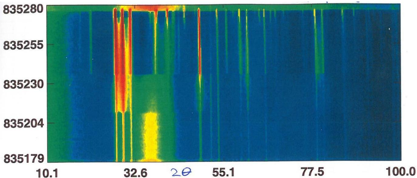
**Figure 2:** Map of diffraction patterns as a function of temperature: No. 835179-210: 90-150 K; no. 835211-234: 160-180 K; no. 835235-280: 185-280 K. Note the broad amorphous feature at ~ 35 deg. which disappears at ~ 150 K.
