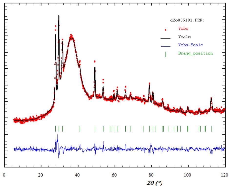
**Figure 1:** Diffraction pattern of hyper-quenched NaCl·10.2D<sub>2</sub>O at 90 K. Peaks are from a small quantity of crystalline D<sub>2</sub>O ice Ih. The line through the data is a Rietveld fit (pattern matching).
