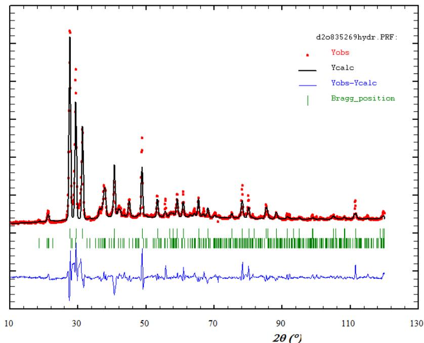
**Figure 4:** Diffraction pattern of glassy  $\text{NaCl}\cdot 10.2\text{D}_2\text{O}$  after recrystallisation, at 250 K. The line through the data is a Rietveld fit assuming ice Ih and the dehydrate  $\text{NaCl}\cdot 2\text{D}_2\text{O}$  [4] (lower tickmarks). Scale factors Ice Ih/hydrate: 114/4.8 ~24.
